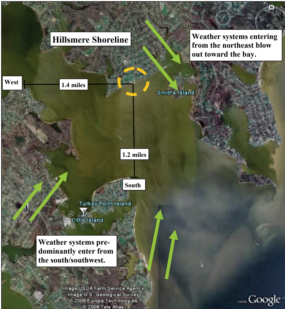
Figure 2. Storms typically enter the state of Maryland from the south/southwest and northeast. Despite the sites long stretches of apparent fetch the area is well protected by features like Turkey Point, shallow shoals, and the southern tip of Hillsmere peninsula. Storms entering from the northeast blow away from the Hillsmere shoreline. The shoreline's northeasterly aspect helps to deflect/dissipate wave energy associated with storms and plays a role in longshore transport.
