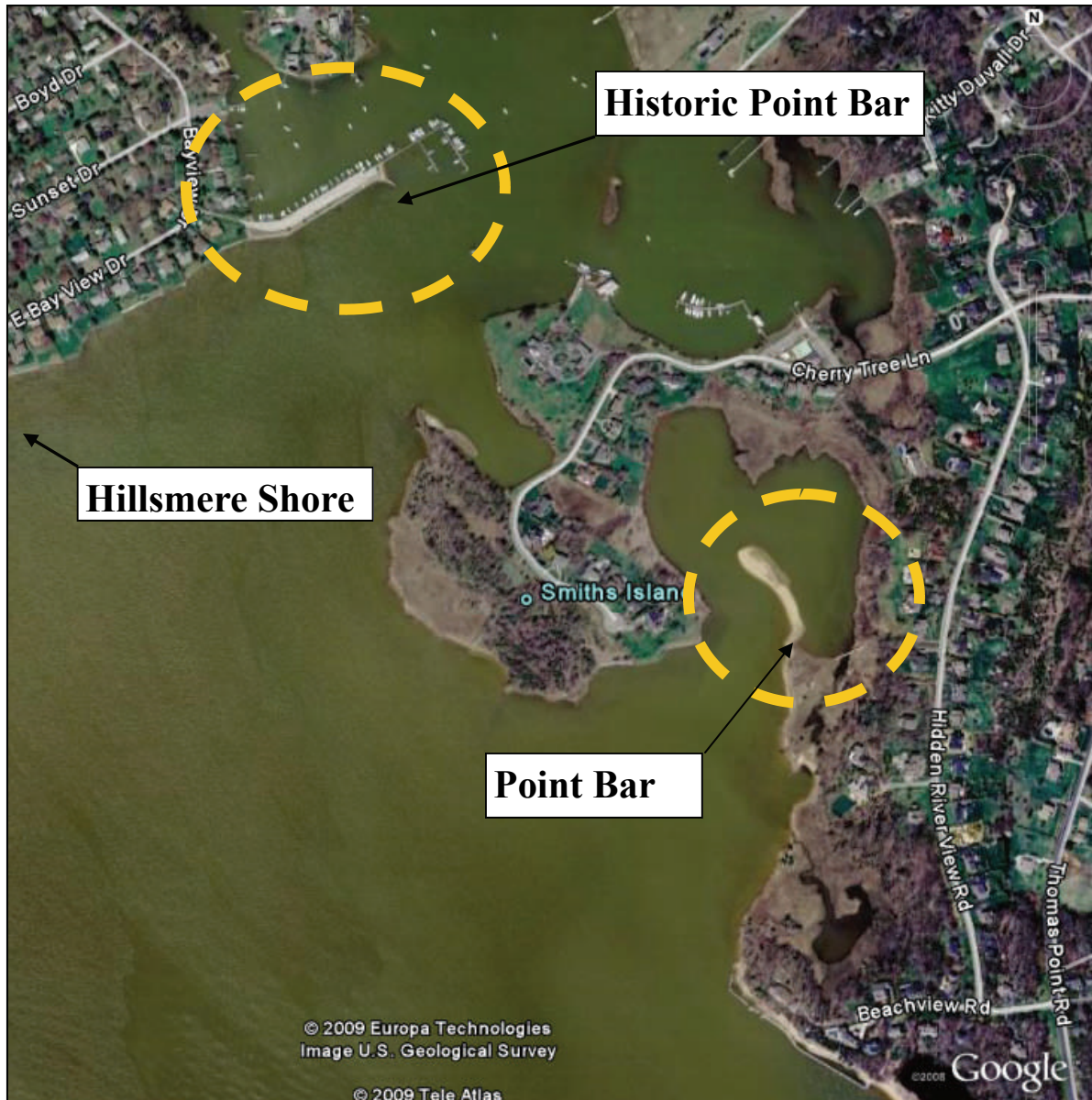
Figure 11. Point bars can result when littoral drift occurs uninhibited by shoreline structures. This point bar is a result of littoral drift accretion in Cherrytree Cove. Historically transport lead to a point bar extending from the shoreline into Duvall Creek. This point bar has since been converted into a marina. The rip-rap bulkheads at Hillsmere inhibit some transport into Duvall Creek.
