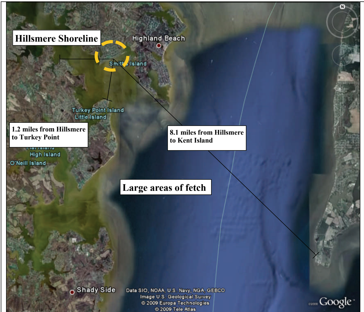
Figure 4. The Hillsmere shoreline initially appears vulnerable during storms due to long stretches of fetch. Storms typically enter the state of Maryland from the south southwest and northeast. The Hillsmere shoreline is actually well protected from storm systems by shallow shoals and protruding land features like Turkey Point.
