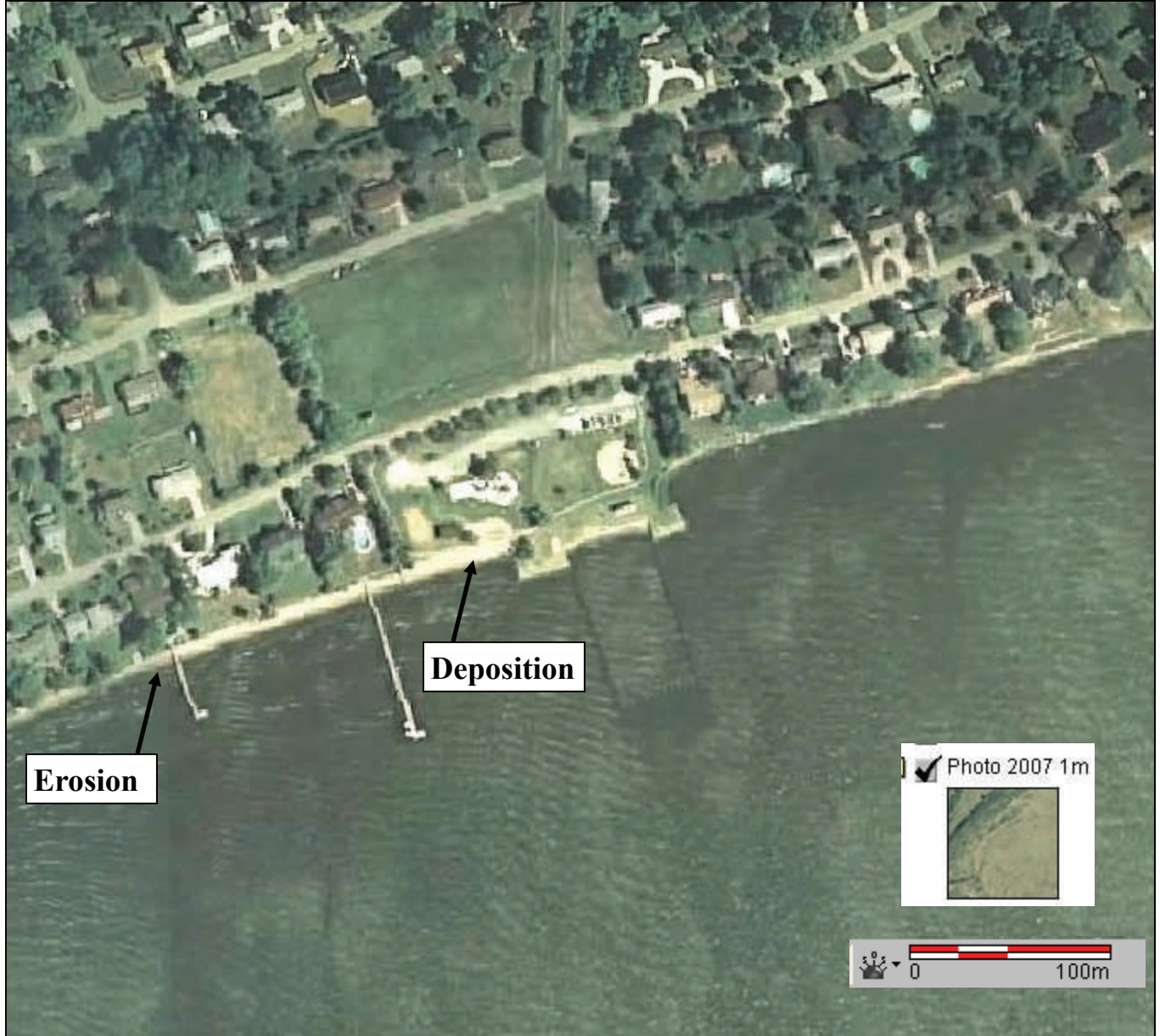
Figure 9. Current erosion and deposition features at Hillsmere Shoreline. Deposition is occurring along the southwest bulkhead. Aerial photo from 2007.
